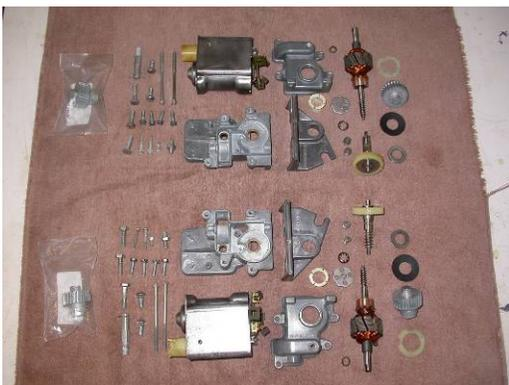
Every article warns about the possibility of the spherical bearing being seized to the armature. Sure enough, both our motors were seized and as a result popped out of their spring retainer.
