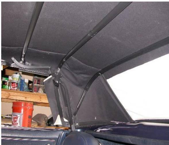
The front header bow had some rust issues, but the rest of the convertible top frame was in good shape. Tim welded in some repairs to the front bow and thoroughly cleaned and sanded the frame. We did not disassemble the frame since it was mostly riveted together. That turned out to be a good choice since it came out looking like new after a coat of semi-gloss black paint.
