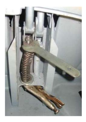
The secured spring will easily go back over the stud and the plastic ties, heater hose and wire can then be removed. Then finish installing the spring. Note the use of the large washer at the base.
