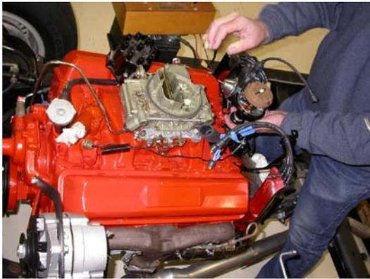
Doug Banner gave the group a demonstration of the proper way to stab a distributor into a recently completed engine. In this case, the engine is a '66 327 and is in David's recently completed rolling chassis. Doug discussed the common mistakes made when installing a distributor, the results, and the remedies.
