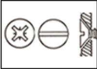
**FLAT HEAD (100' COUNTERSUNK):** This special flat head screw has been developed for applications requiring flush surfaces, and is recommended for use in soft materials. To distribute pressure over a larger and less angular surface. Very well adapted for use with thin aluminum, soft plastics, etc.
